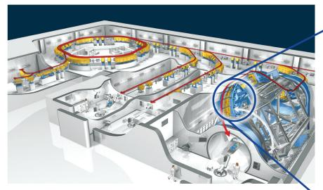
The HIT ion therapy centre in Heidelberg Germany has been treating patients since 2009. It is the only one among the European ion therapy centres to operate a gantry which is 19 m long, and about 15 m in diameter. The total weight is 600 tons. Current studies show that the weight of the SEEIIST gantry could be reduced by about a factor ten.
